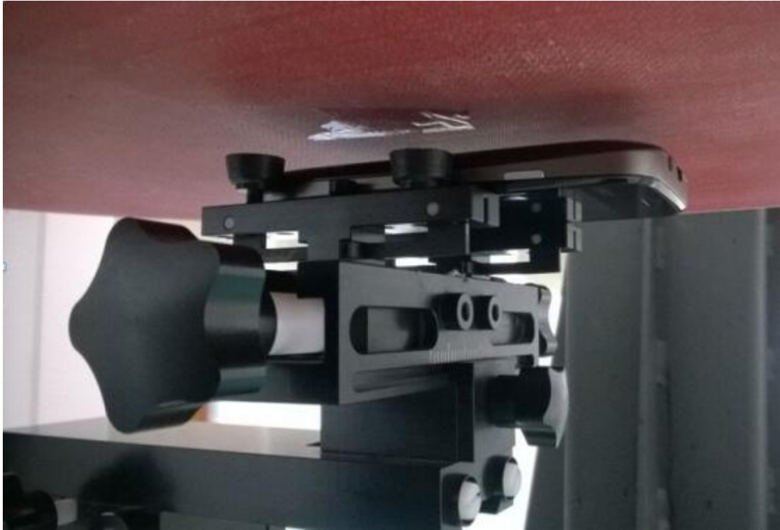
Pic5.Body SAR Back to the phantom (10mm)
