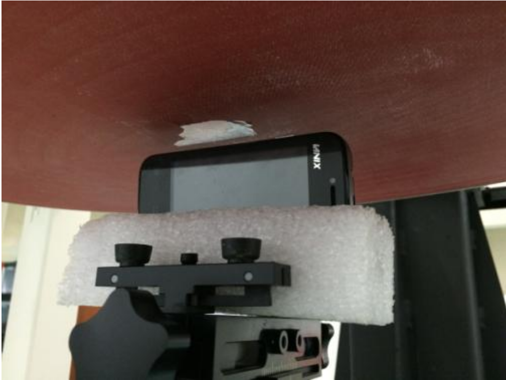
Pic7.Body SAR Left to the phantom (10mm)
