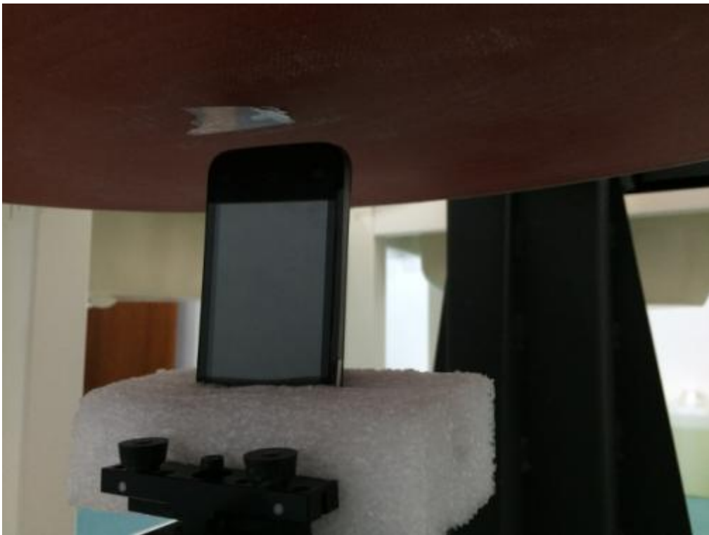
Pic10.Body SAR Bottom to the phantom (10mm)
