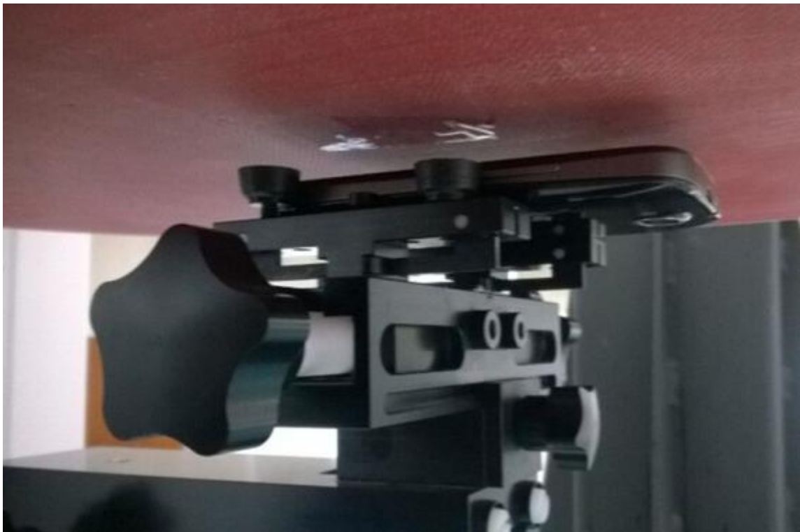
Pic6.Body SAR Face to the phantom (10mm)
