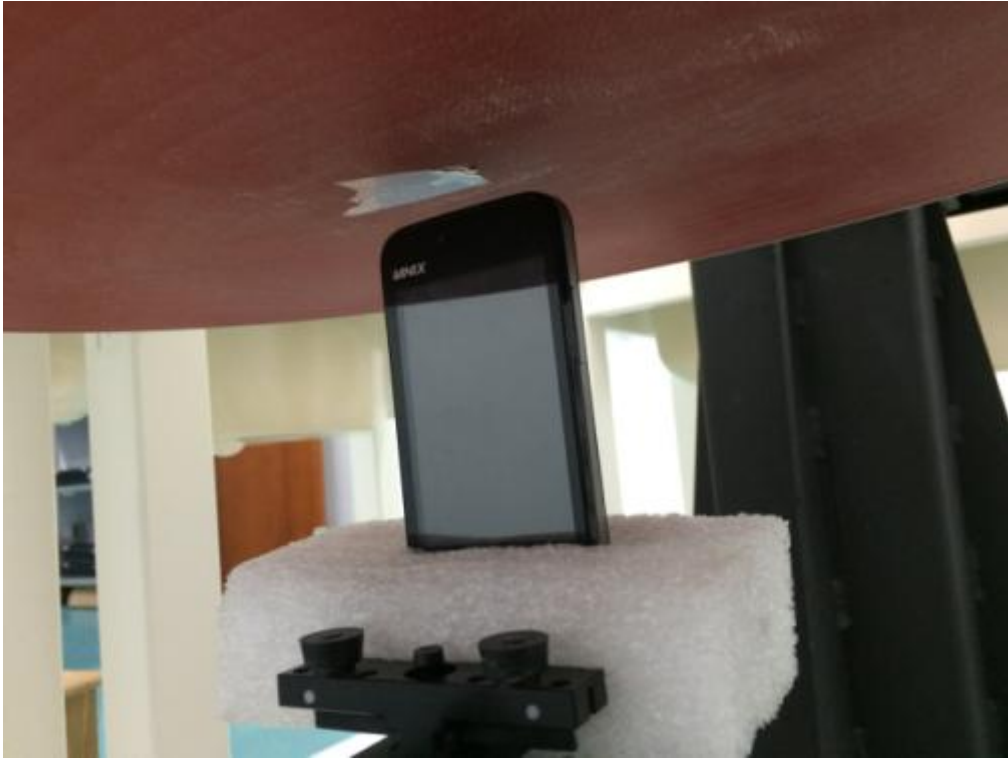
Pic9.Body SAR Top to the phantom (10mm)
