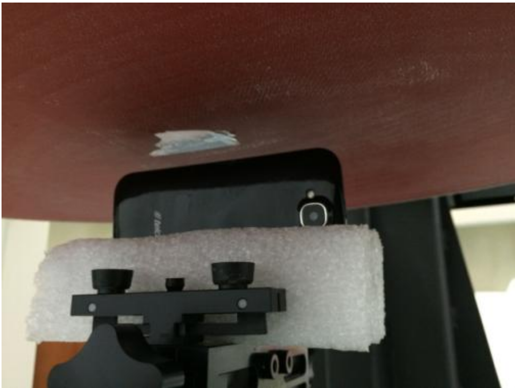
Pic8.Body SAR Right to the phantom (10mm)
