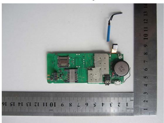
3. Mainboard rear view with shielding
