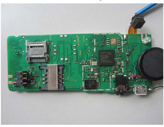
4. Mainboard front view without shielding
