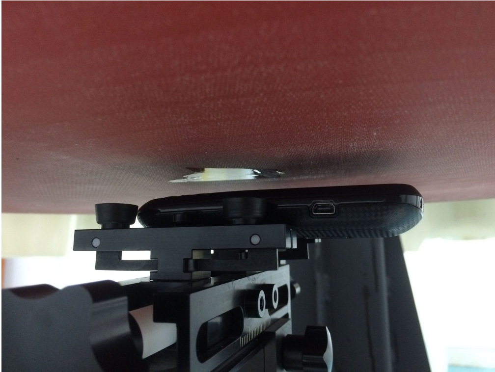
Pic5.Body SAR Back to the phantom (10mm)
