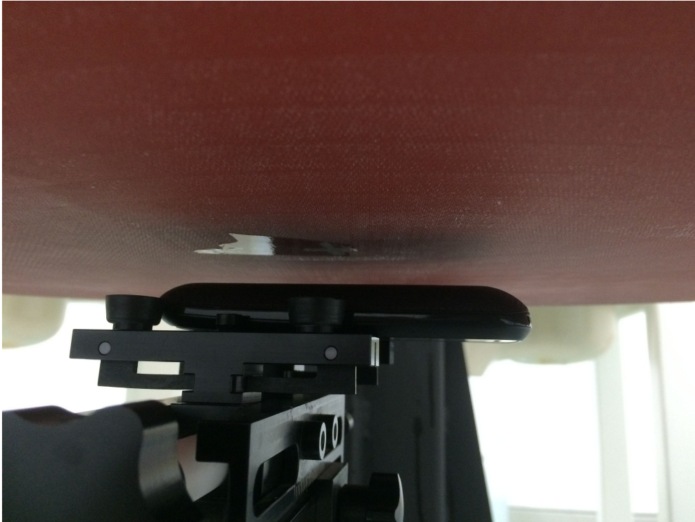
Pic6.Body SAR Face to the phantom (10mm)
