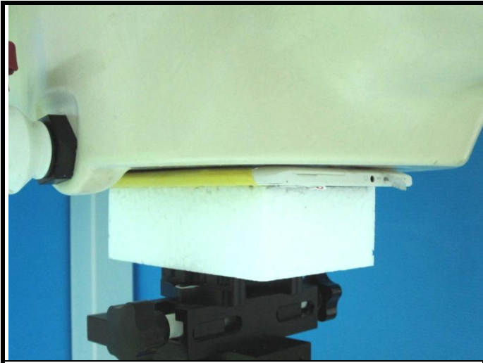
Rear Face of EUT with 0 cm Gap
