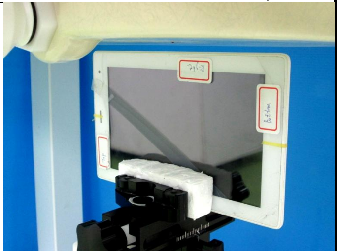
Right Side of EUT with 0.7 cm Gap
