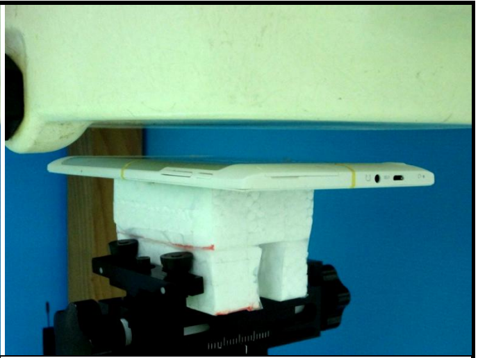
Rear Face of EUT with 1.8 cm Gap
