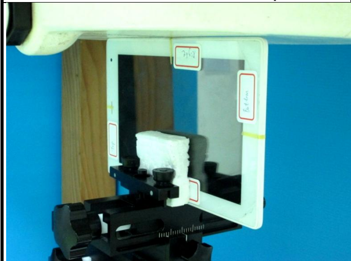
Right Side of EUT with 0 cm Gap
