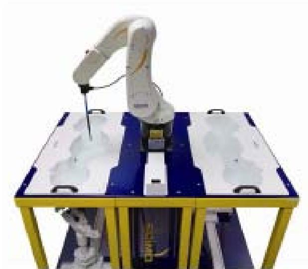
The EUT under test operating at the maximum power level is placed in the phone holder, under the phantom, which is filled with head simulating liquid. The E-Field probe measures the electric field inside the phantom. The OpenSAR software computes the results to give a SAR value in a 1g or 10g mass.
