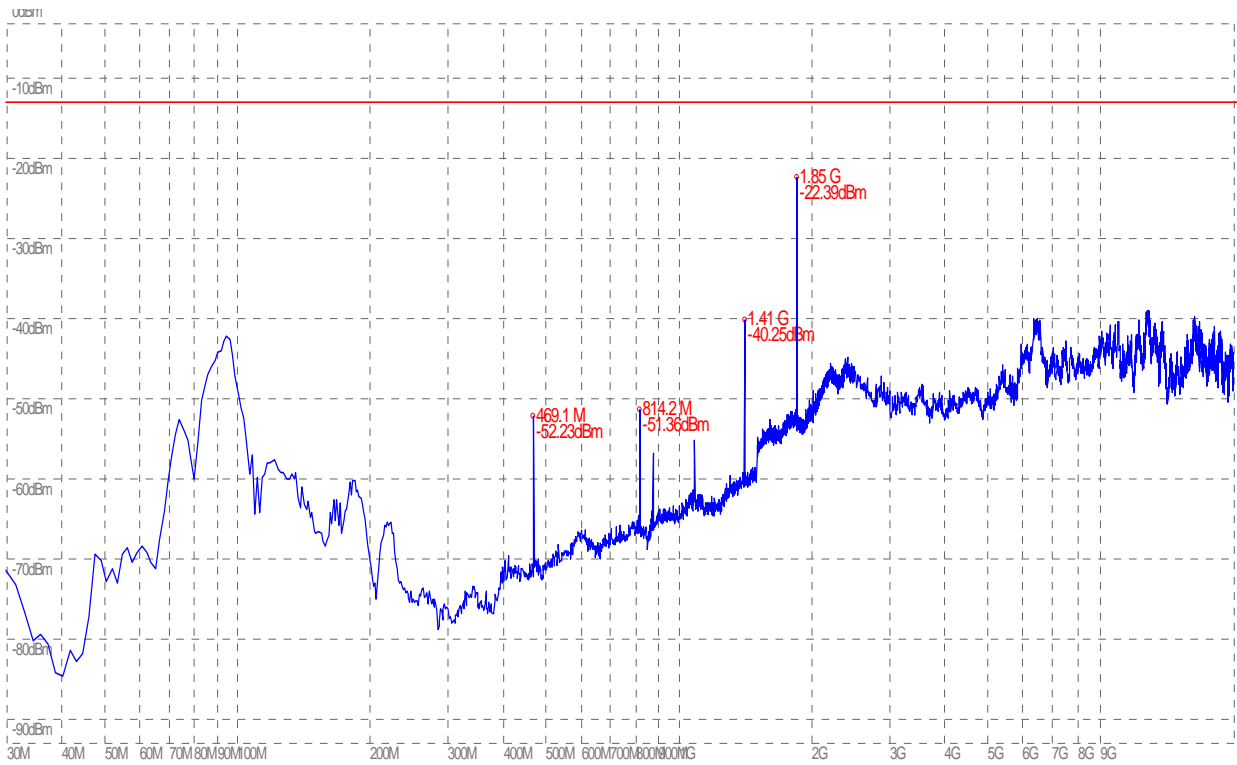
(Plot B.1: GSM 1900MHz Channel = 512, Test Antenna Horizontal)
