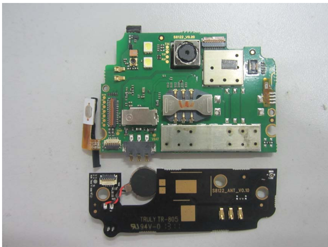
2. Mainboard front view with shielding
