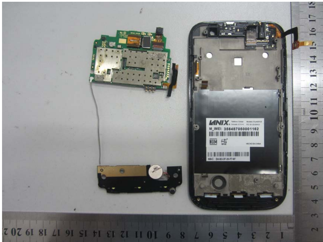
2. Mainboard front view with shielding
