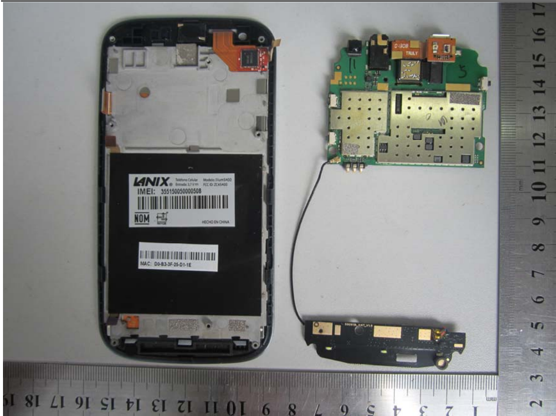
2. Mainboard front view with shielding
