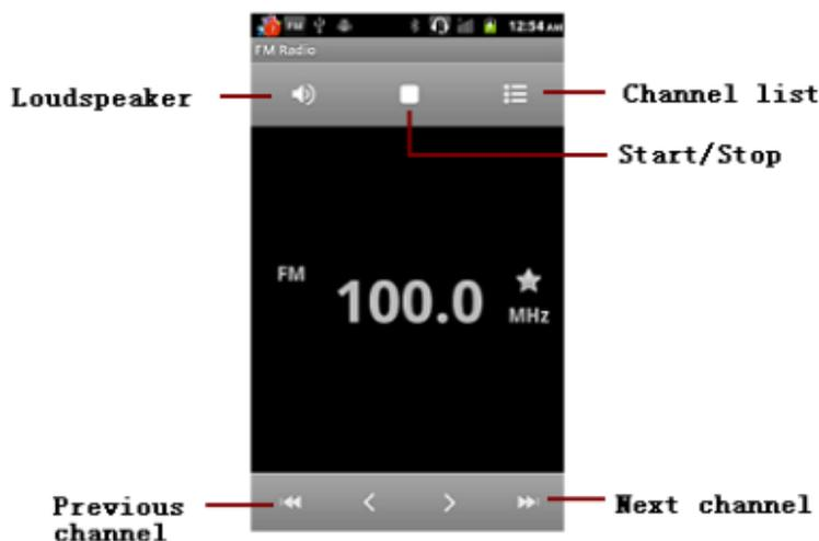
Attention: this handset doesn't have a built-in antenna. If you want to listen to the radio, please insert the headphone first. Pressing the side key can adjust the volume.
