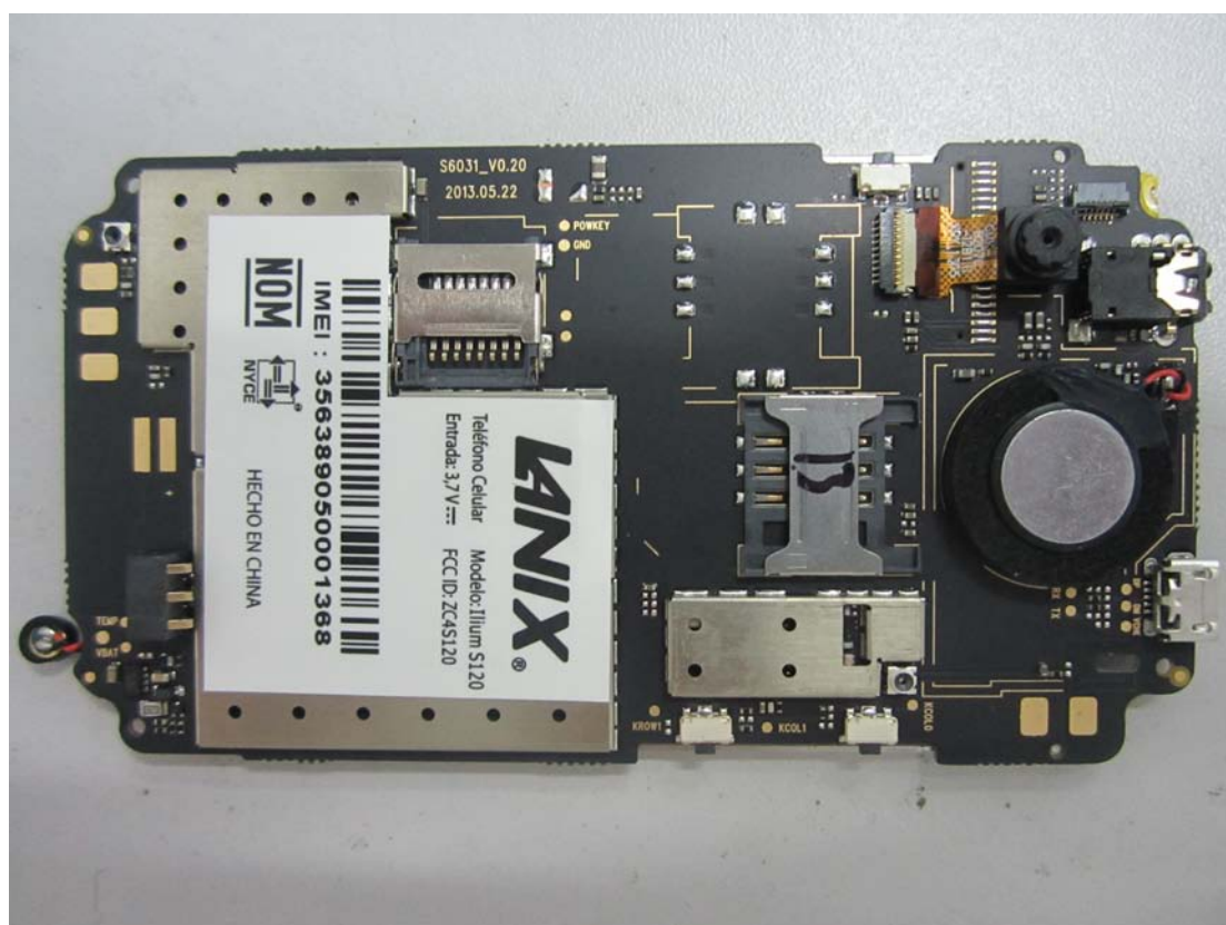
2. Mainboard front view with shielding
