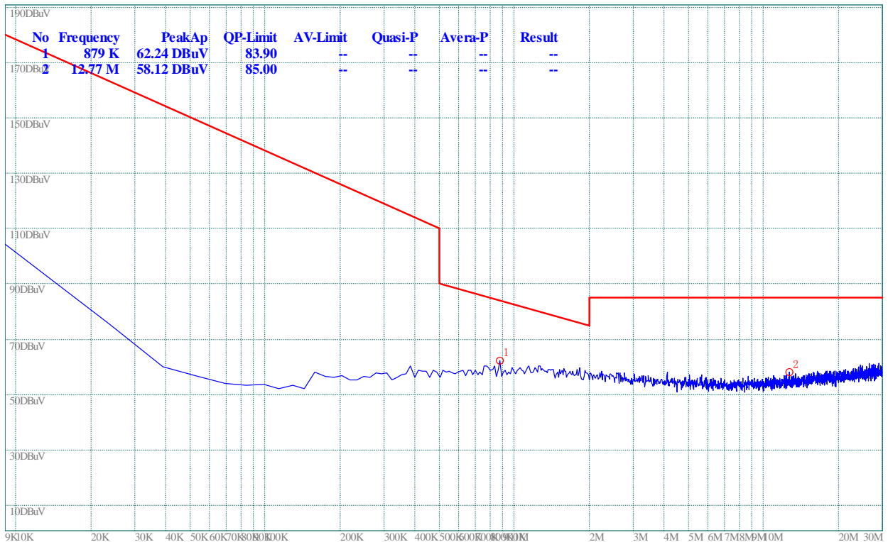
(Plot C.0: 9kHz to 30MHz @ 8-DPSK, channel 78)
