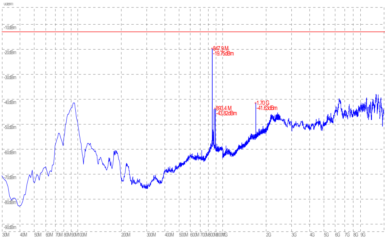
(Plot C.5: EGPRS 850MHz Channel = 251, Test Antenna Horizontal)
