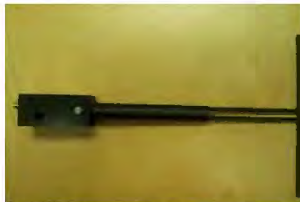
Figure 1 – MVG COMOSAR Validation Dipole
