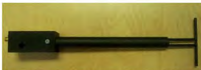
Figure 1 – MVG COMOSAR Validation Dipole
