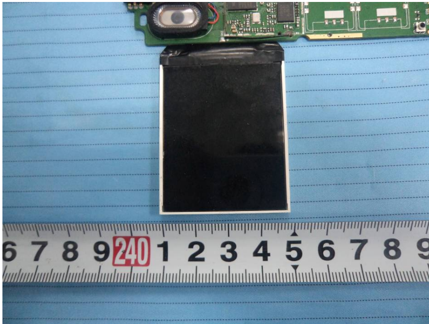
EUT – LCD Top View
