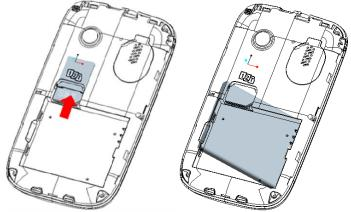
**Warning:** Make sure to switch off the phone before taking out SIM card, otherwise your SIM card might be damaged.
