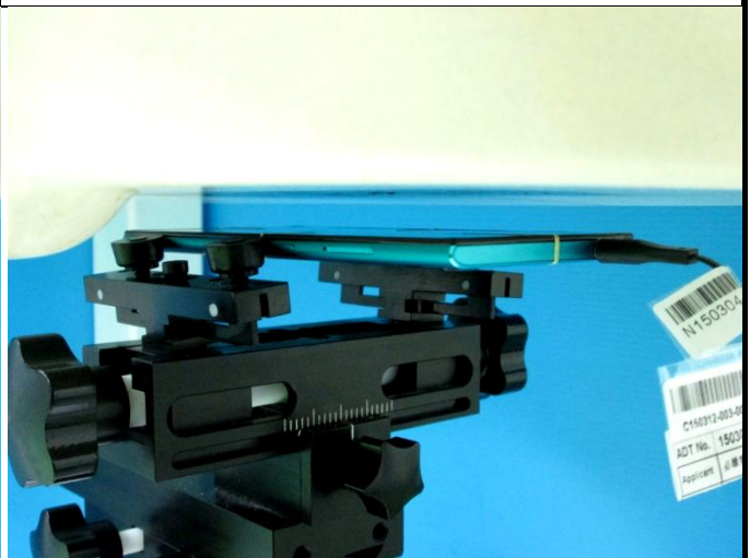
Front Face of EUT with 1.0 cm Gap (with Earphone)
