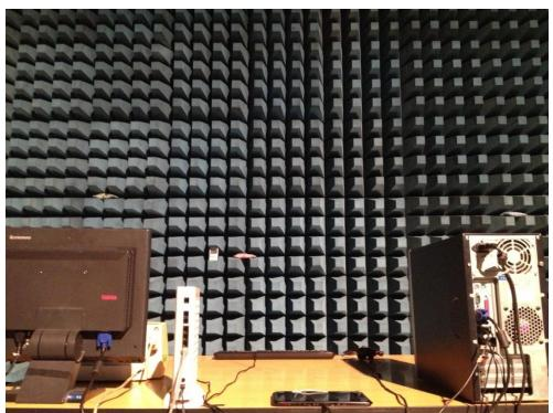
FCC Part15B Radiated Emission above 1GHz Setup 1- EUT+ Battery +PC+ LCD monitor -Front
