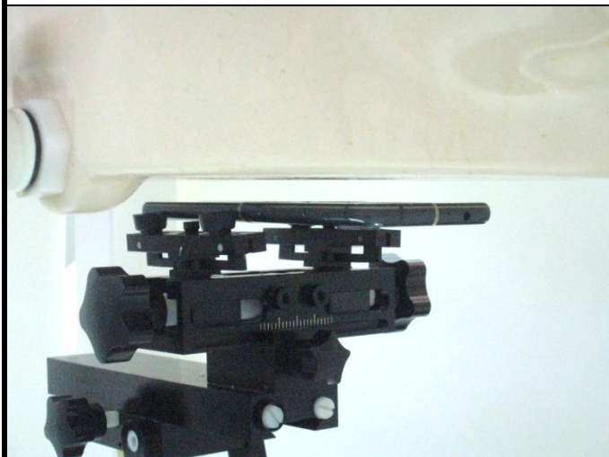
Front Face of EUT with 1.0 cm Gap
