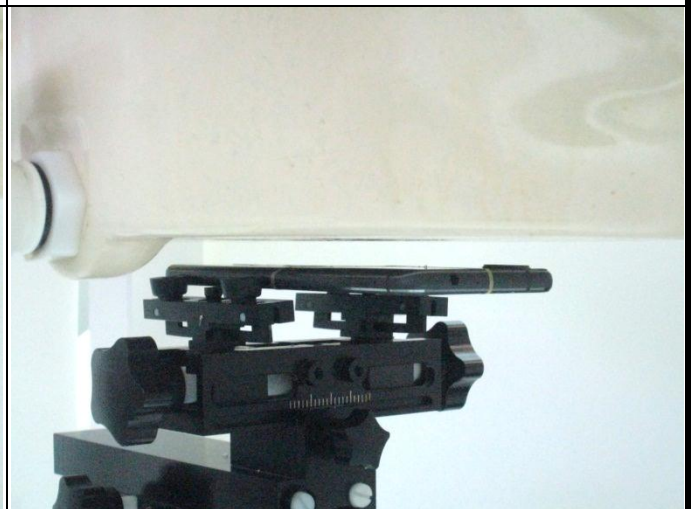
Rear Face of EUT with 1.0 cm Gap
