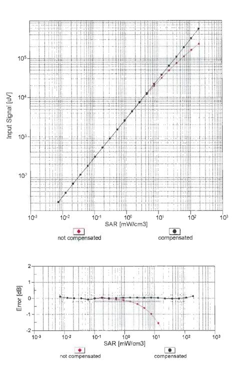
Dynamic Range f(SAR<sub>head</sub>) (TEM cell , f<sub>eval</sub>= 1900 MHz)
