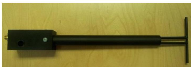
Figure 1 – MVG COMOSAR Validation Dipole
