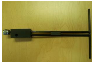
Figure 1 – MVG COMOSAR Validation Dipole
