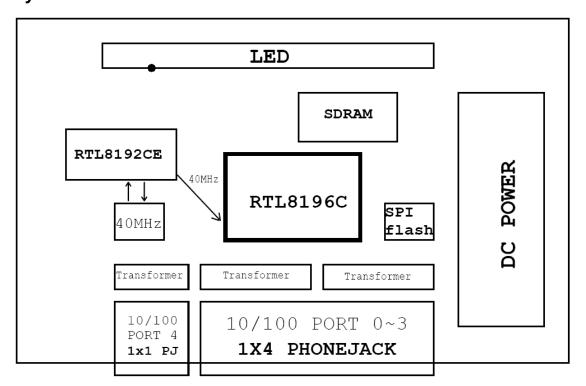
The RTL8196C integrates a media access control (MAC), a baseband processor, analog-to-digital and digital-to-analog converters, USB2.0 client controller and transceiver in one package.
