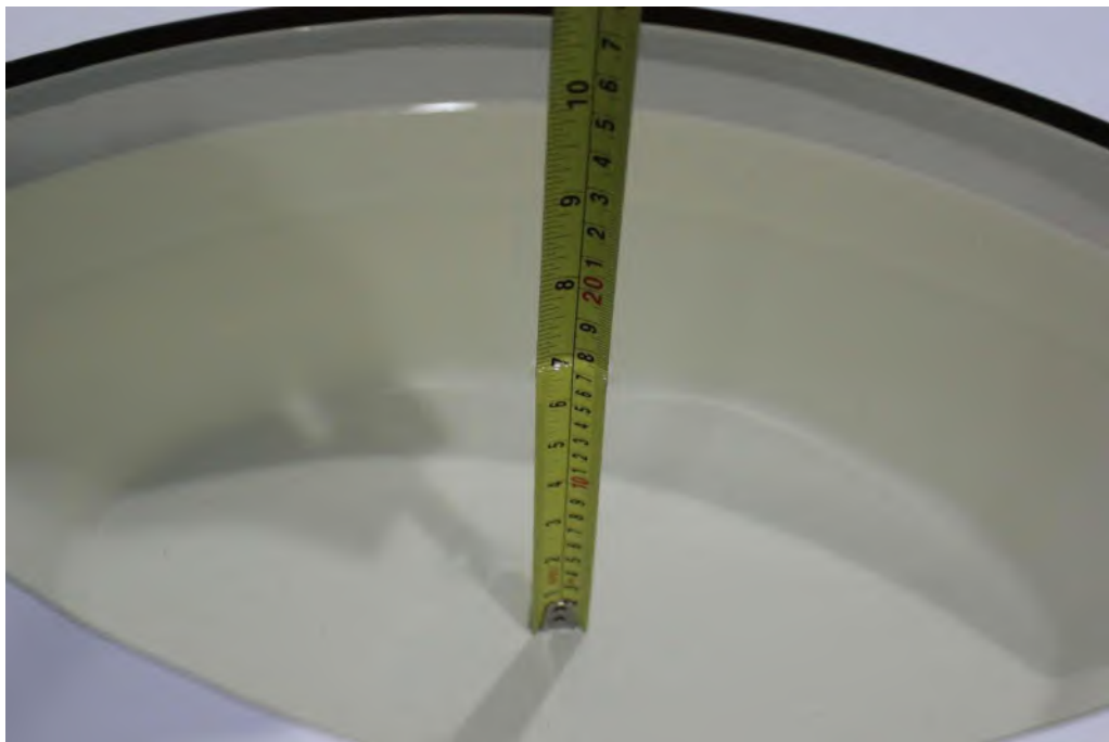
Picture 7-6: Liquid depth in the Flat Phantom(5GHz)
