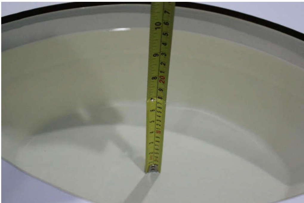
Picture 7-6: Liquid depth in the Flat Phantom(5GHz)
