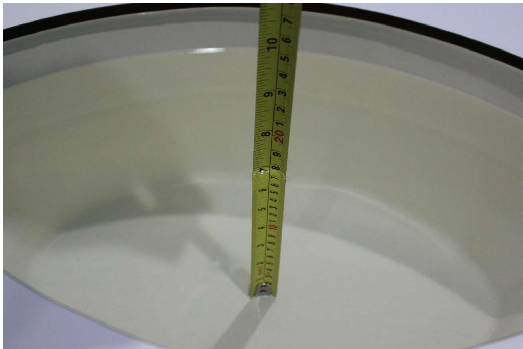
Picture 7-6: Liquid depth in the Head Phantom(5GHz)
