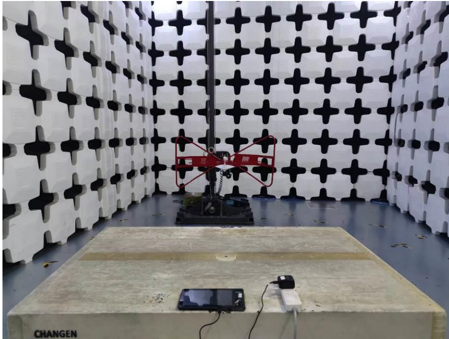
9. Radiated Emissions (Part 15B, Camera,30MHz-1GHz)
