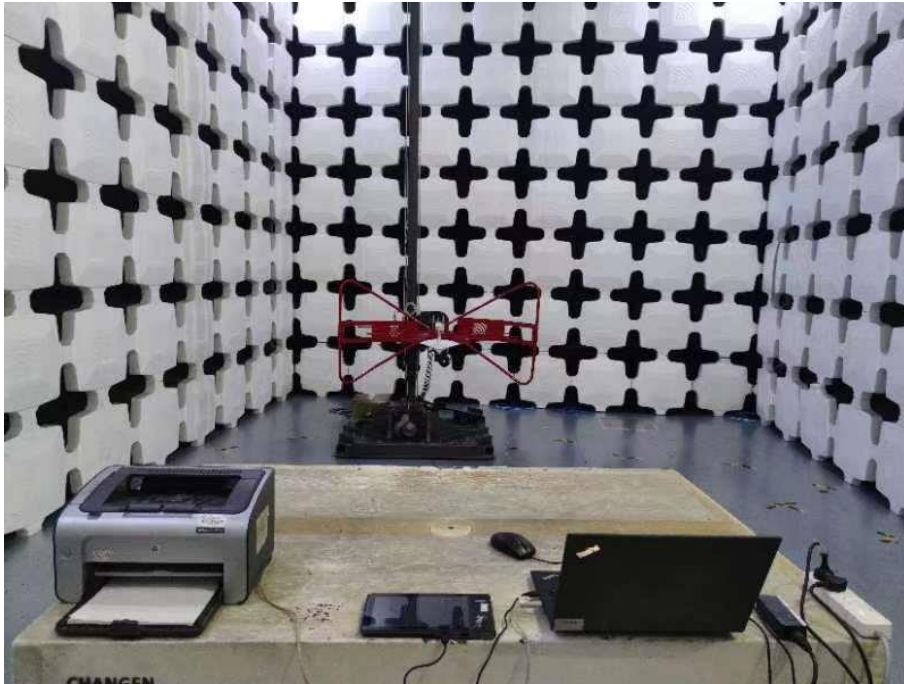
1. Radiated Emissions (Part 15B, Data Transfer,30MHz-1GHz)
