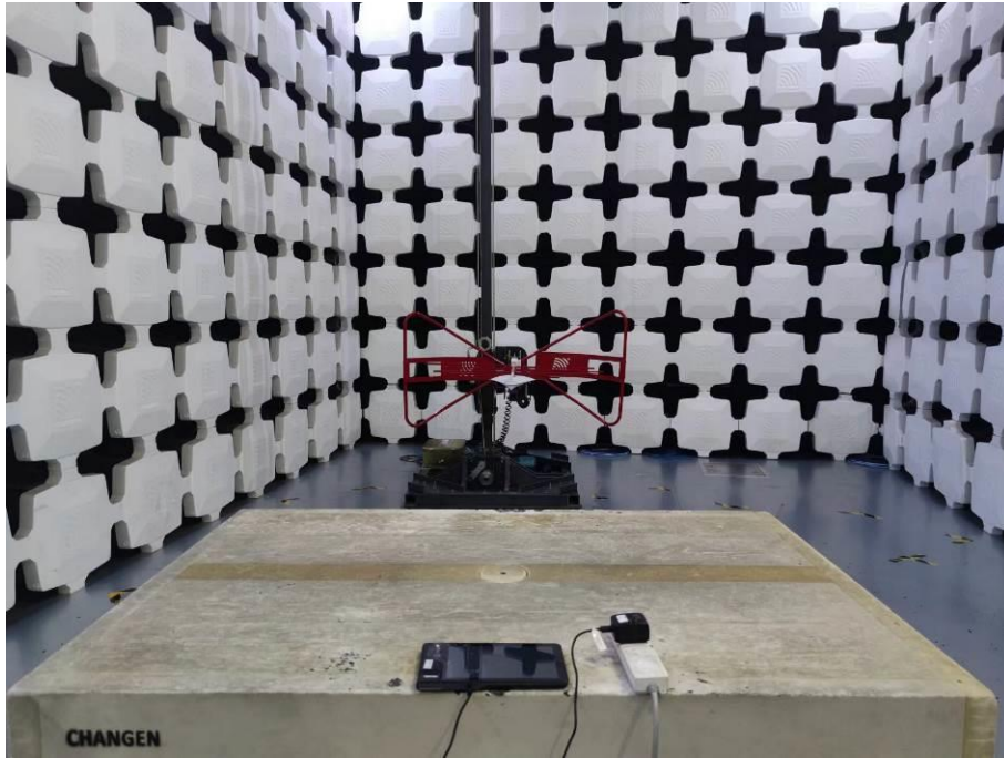
5. Radiated Emissions (Part 15B, Camera,30MHz-1GHz)
