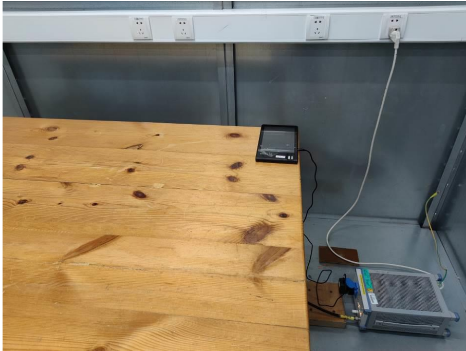
13. Conducted Emission (Part 15B, Camera)
