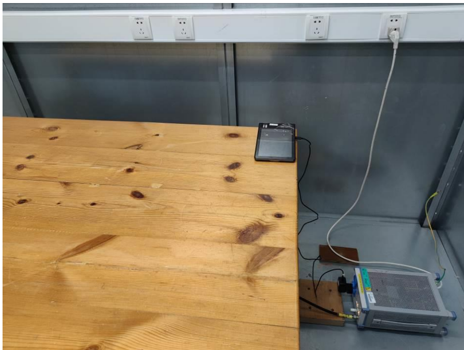
14. Conducted Emission (Part 15B, Camera)
