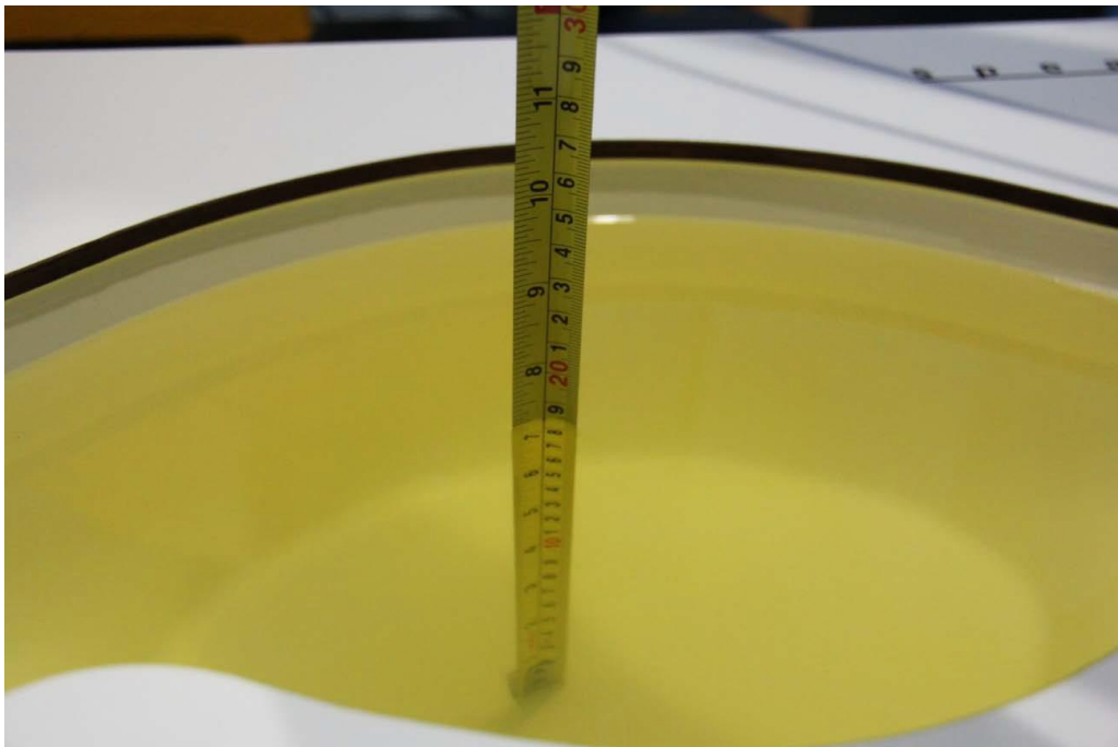
Picture 7-4: Liquid depth in the Head Phantom(2450MHz)
