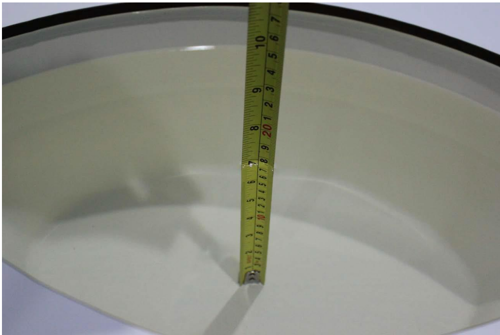
Picture 7-6: Liquid depth in the Head Phantom(5GHz)
