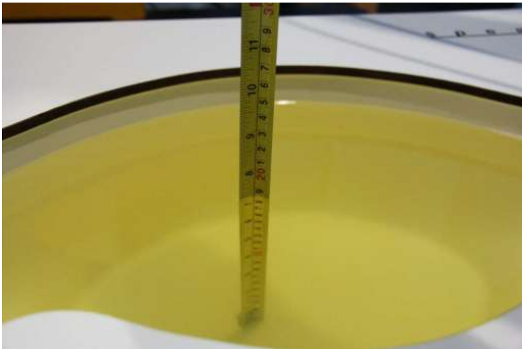
Picture 7-4: Liquid depth in the Head Phantom(2450MHz)
