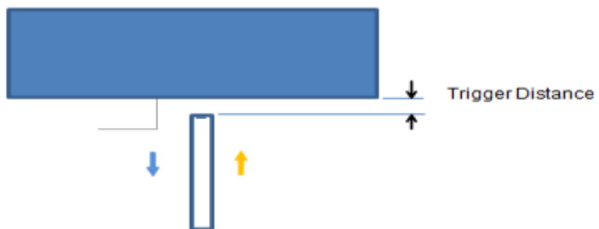
Picture: Proximity sensor triggering distances assessment (Tops)
