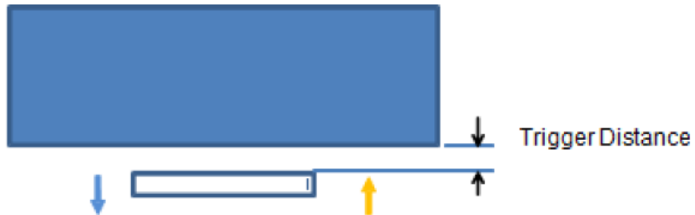
Picture: Proximity sensor triggering distances assessment (Back)
