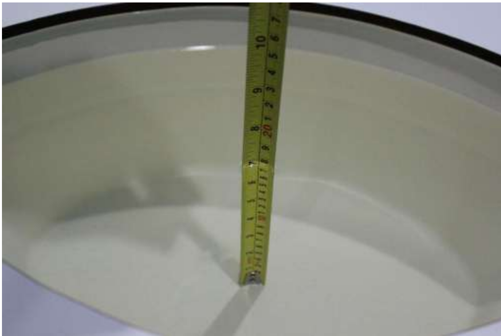
Picture 7-6: Liquid depth in the Head Phantom(5GHz)
