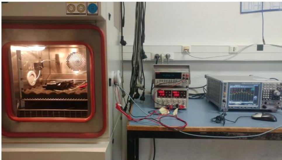
Photo of 20dB emission bandwidth
