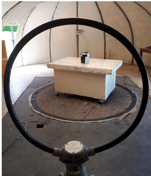
Photograph for Field strength outside of the bands 13.110-14.010 MHz
