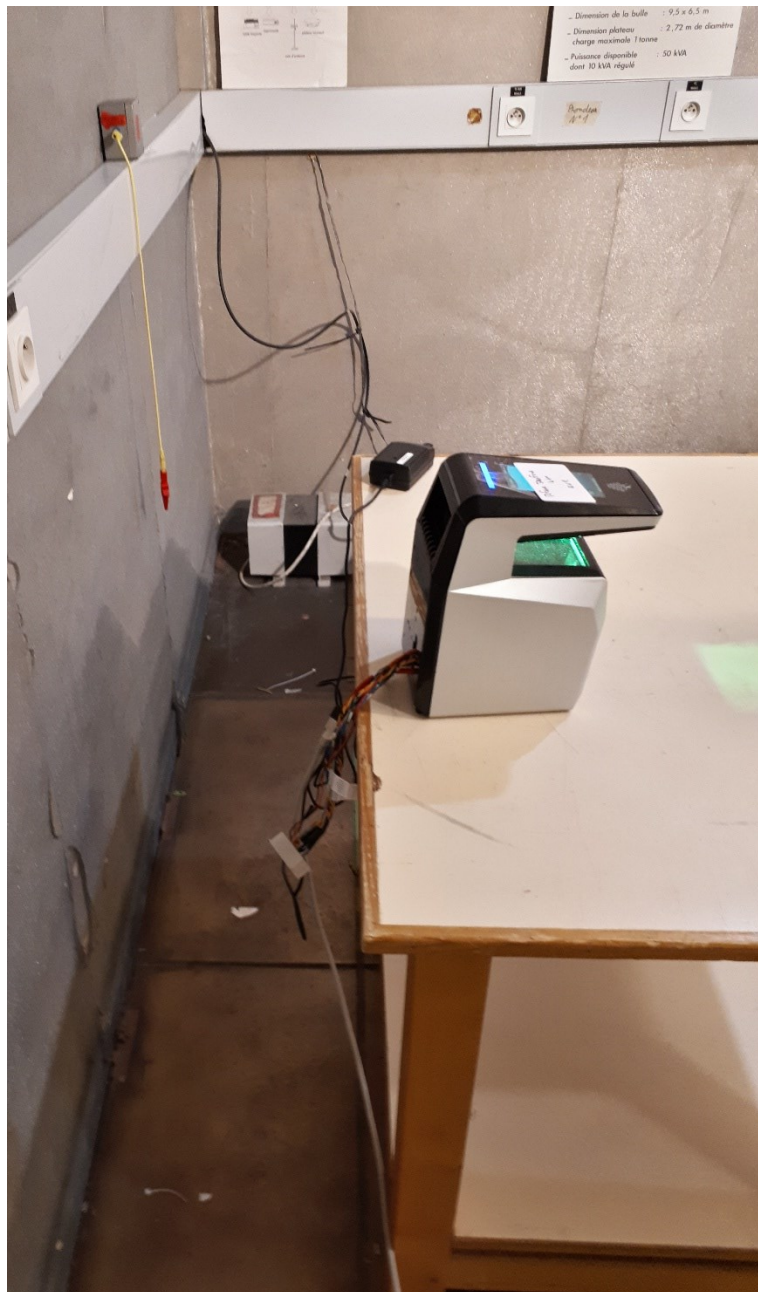
Photograph for AC Power Line Conducted Emissions (Rear view) with DC power supply
