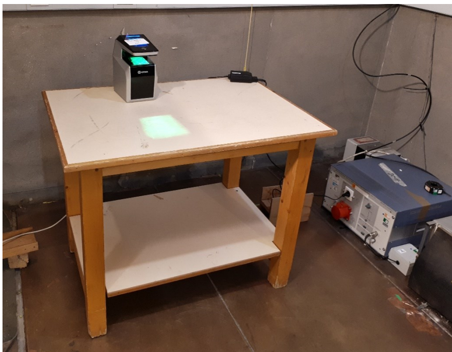
Photograph for AC Power Line Conducted Emissions (Front view) with DC power supply
