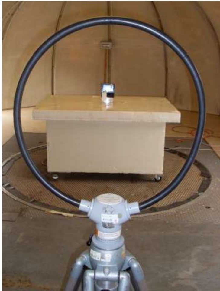
Test setup for radiated field strength
