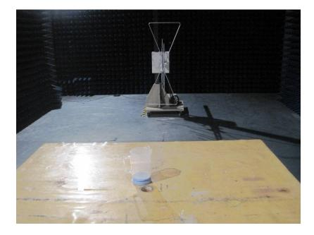
**Radiation Emission Test View For 1GHz-25GHz**
