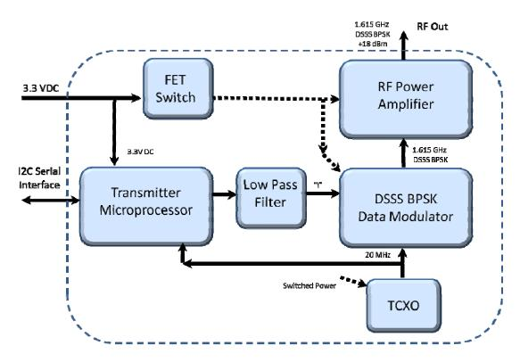
The MYTE module contains a microprocessor that controls the transmitter functions, provides power management and controls the RF transmitter functions. The MYTE module switches the input DC power to create the voltages necessary to minimize power and manage the transmit function.
