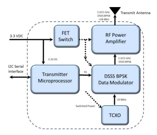
The MYTE module contains a microprocessor that controls the transmitter functions, provides power management and controls the RF transmitter functions. The MYTE module switches the input DC power to create the voltages necessary to minimize power and manage the transmit function.
