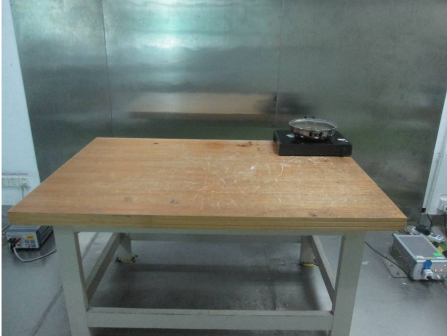
Conducted Emissions - Front View
