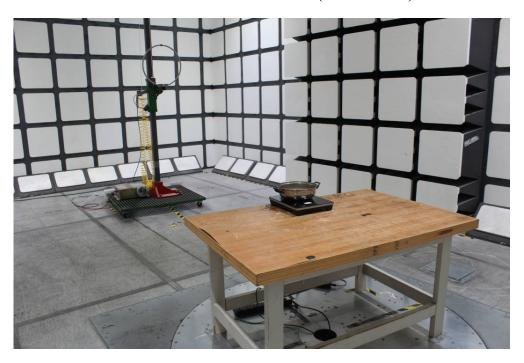
Radiated Emissions – Rear View (9 kHz-30MHz)
