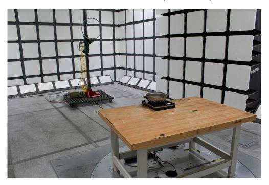
Radiated Emissions – Rear View (9 kHz-30MHz)
