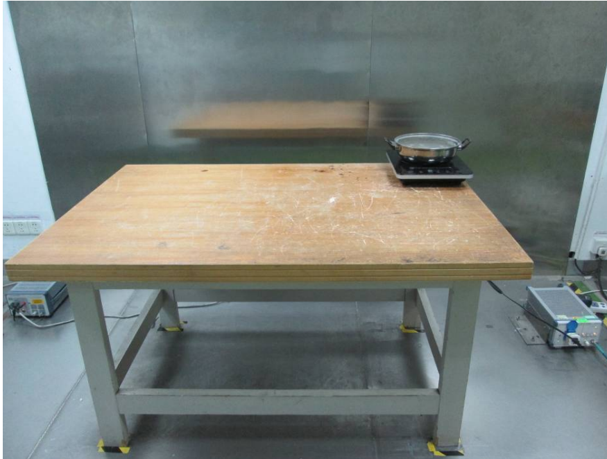
Conducted Emissions - Front View
