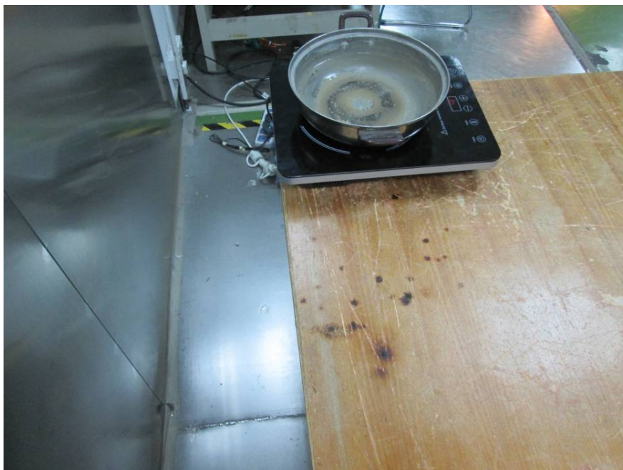
Conducted Emissions - Side View
