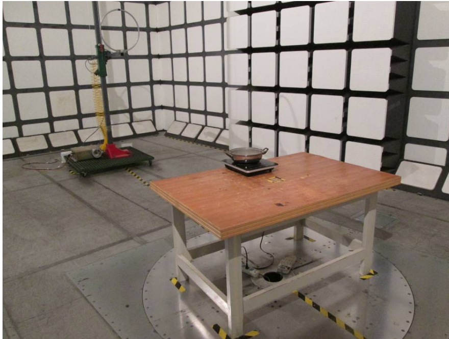
Radiated Emissions - Front View (90 kHz-30 MHz)
