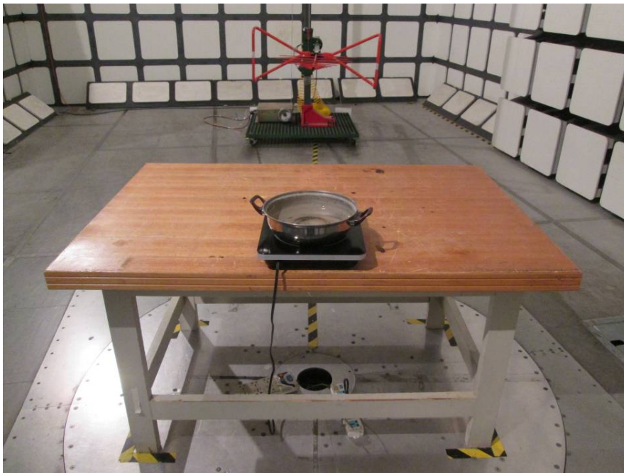
Radiated Emissions - Rear View (30 MHz-1GHz)
