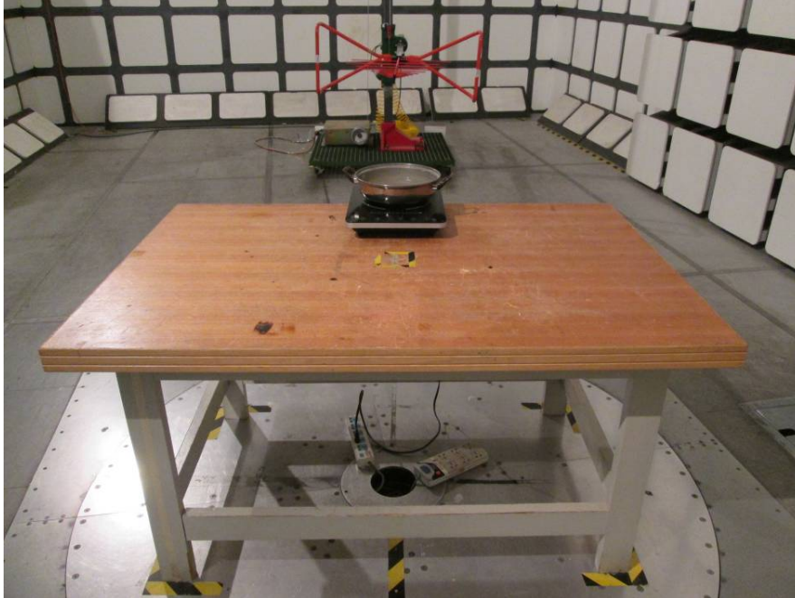
Radiated Emissions - Front View (30 MHz-1GHz)
