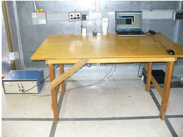
Figure 4.2.4-1: Conducted Emissions Test Setup – Front View
