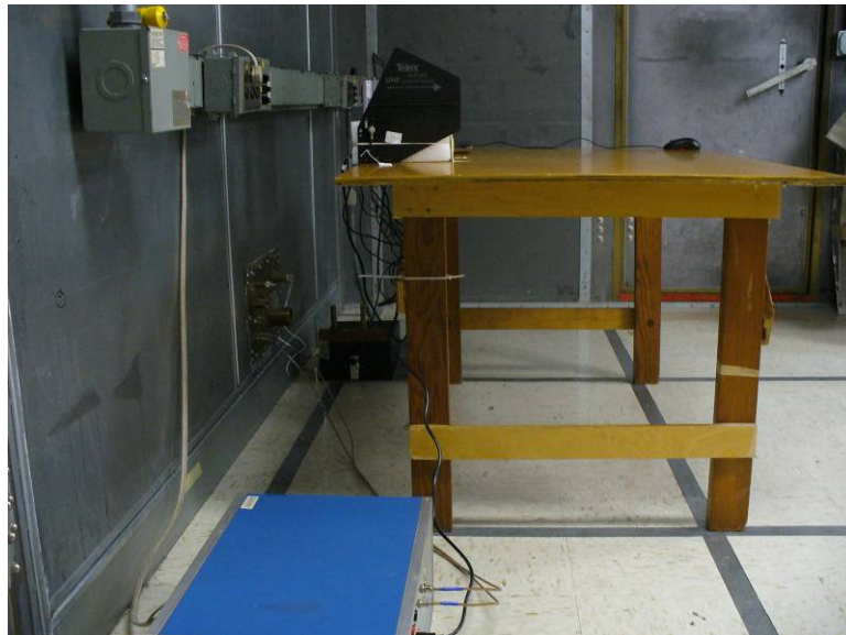
Figure 4.2.4-2: Conducted Emissions Test Setup – Side View
