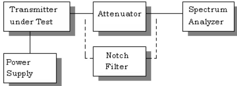
**METHOD OF MEASUREMENT:** The procedure used was ANSI/TIA 603-C:2004. The measurements were made at TIMCO ENGINEERING INC. 849 N.W. State Road 45, Newberry, Florida 32669.
