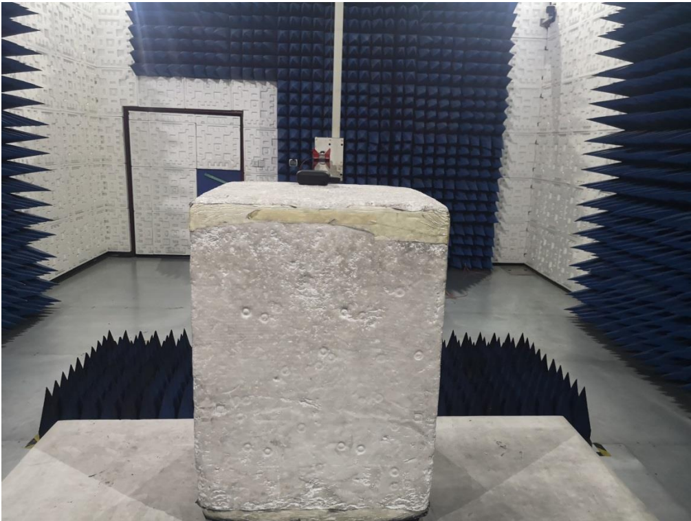
RADIATED EMISSION TEST SETUP ABOVE 1GHz
