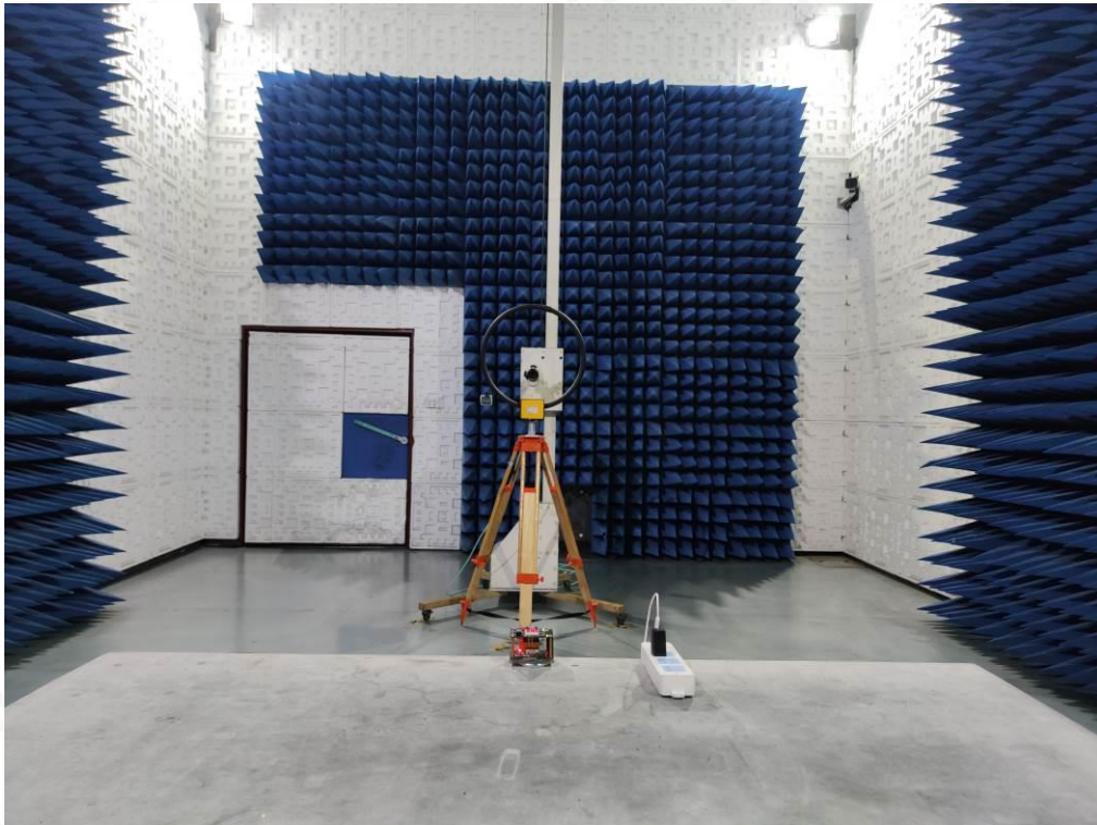
FCC RADIATED EMISSION TEST SETUP 30MHz-1GHZ
