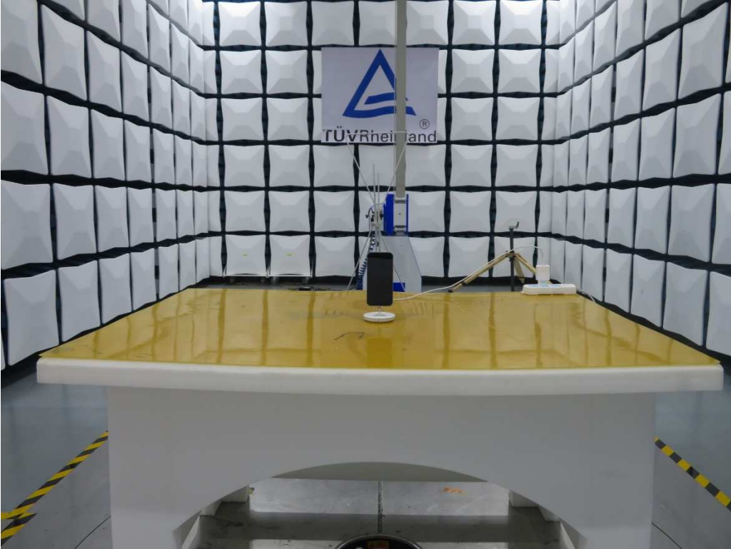
Photograph 2: Set-up photo for Radiated Spurious Emission, 30MHz - 1GHz For Apple Magsafe:
