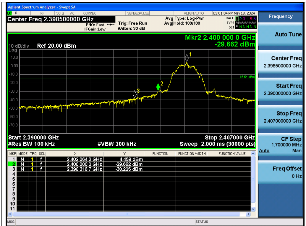
Test_Graph_LE2M_ANT1_2402_2Mbps_Lower Band Edge Emissions
