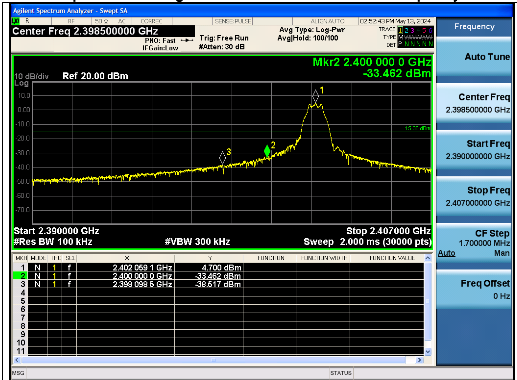
Test_Graph_LE1M_ANT1_2402_1Mbps_Lower Band Edge Emissions
