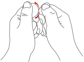
Use the warping provided with the package, find the slot, use the rounded end, push against one side to the other side, you can open the battery box.
