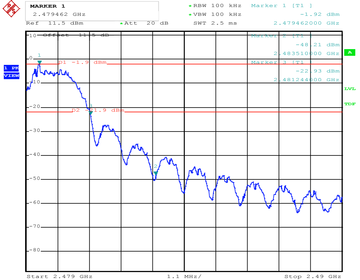
Figure 13: Band Edge Conducted Emission, Spectral Diagram, Mode C (2480MHz)
