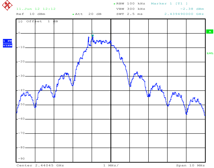
Figure 10: Power Spectral Density, Mode B (2440MHz)
