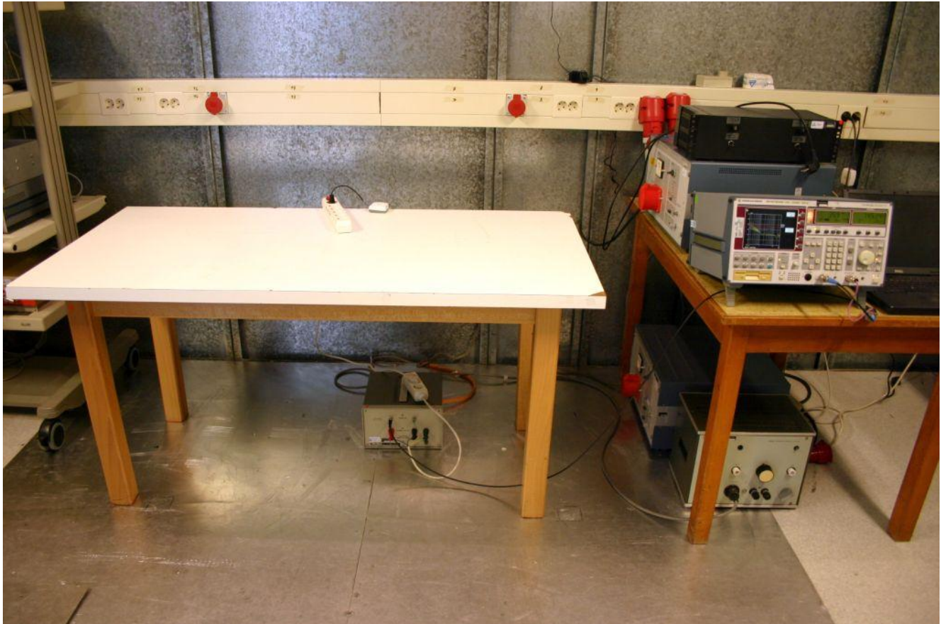
Photo . Basic test set-up conducted emission
