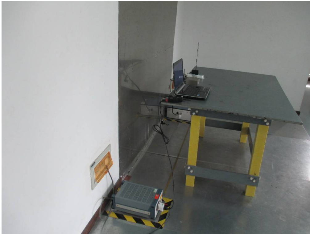
Conducted Emissions Test Setup - Side View
