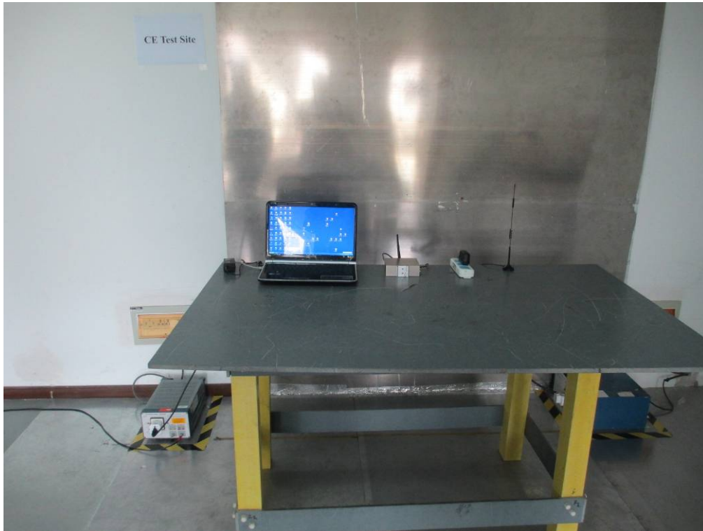
Conducted Emissions Test Setup - Front View
