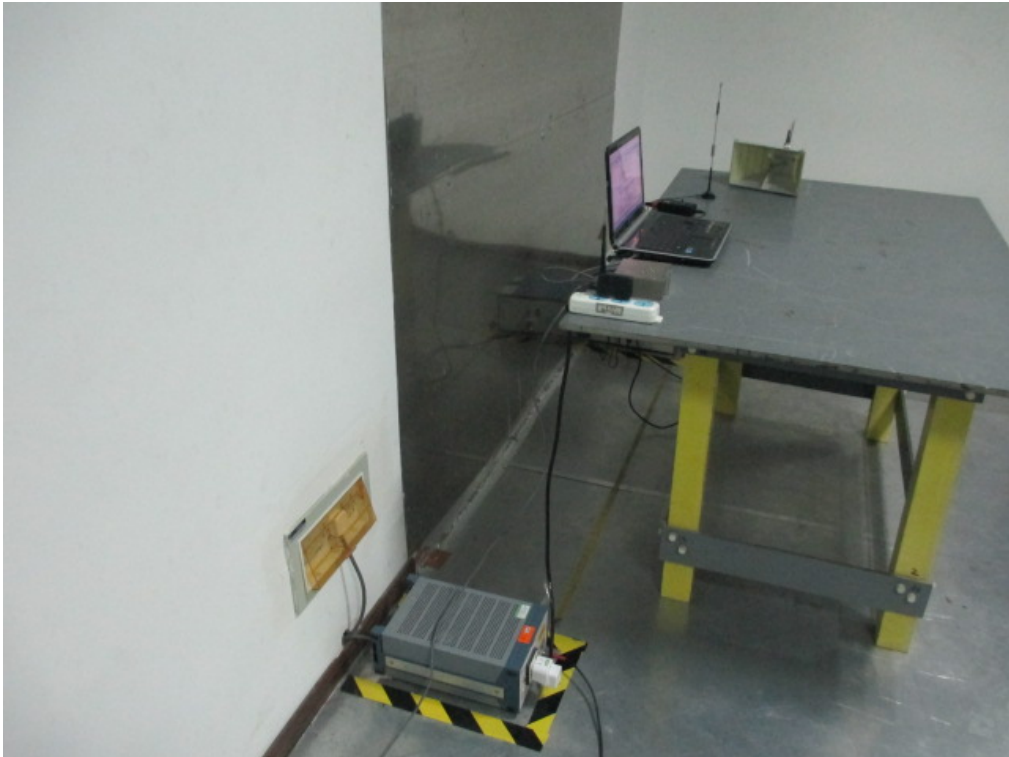
Conducted Emissions Test Setup - Front View
