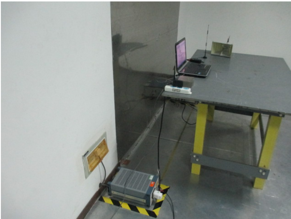
Conducted Emissions Test Setup - Side View
