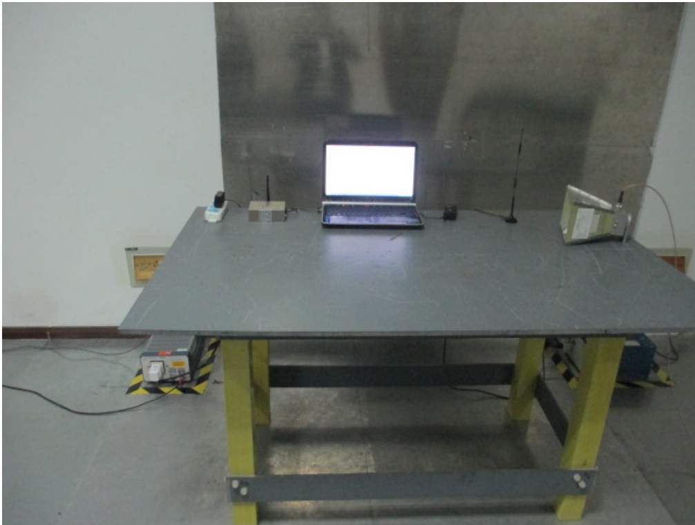
Conducted Emissions Test Setup - Front View
