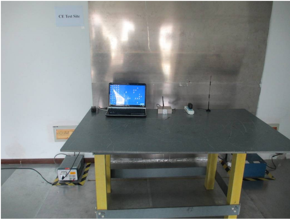
Conducted Emissions Test Setup - Front View
