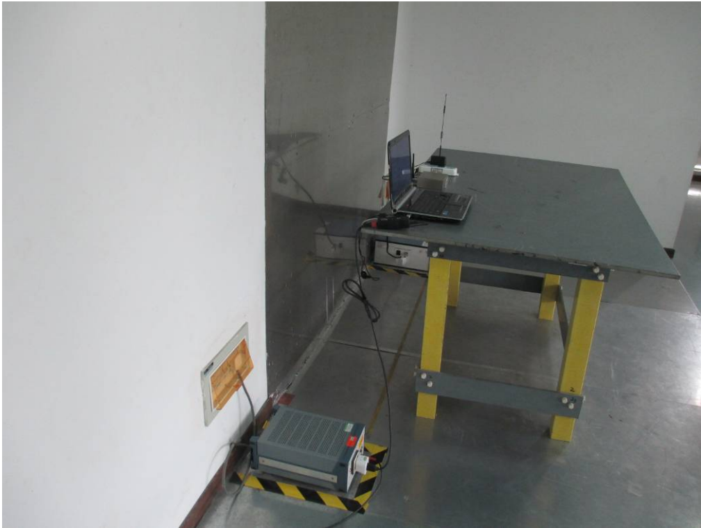
Conducted Emissions Test Setup - Side View
