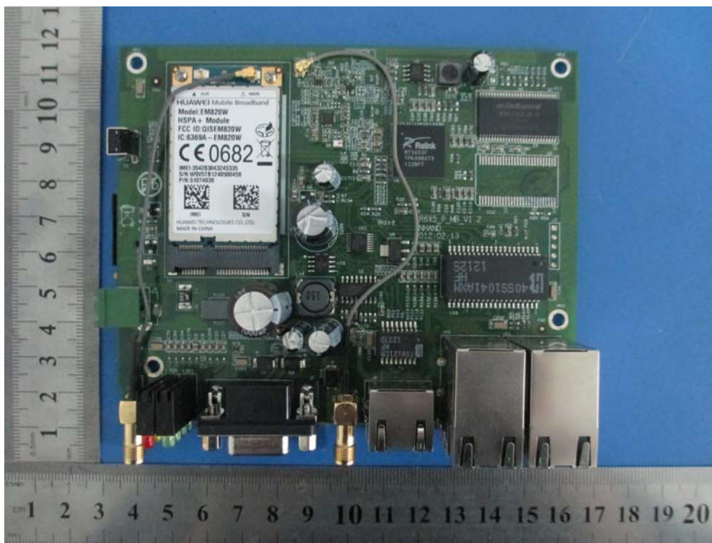
Main Board Front View
